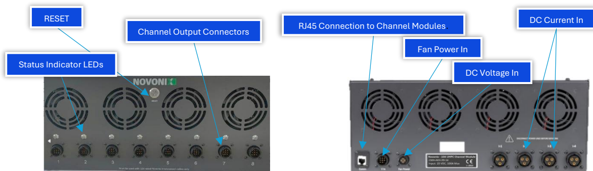
Figure 8: 10A Channel Module front and rear panel I/O scheme
