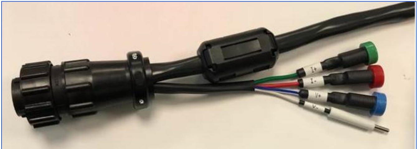
Figure 63: UHPC 2A/10A interconnect cable with Gamry connectors
