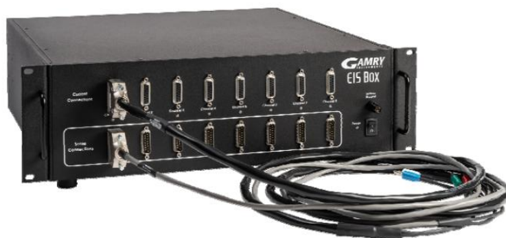
Figure 60: Gamry EIS Box front panel with cell cable attached
