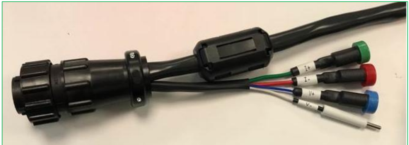
Figure 63: UHPC 2A/10A channel cable with Gamry connectors
